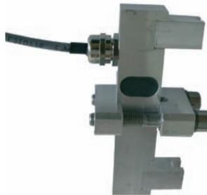
This tensiometer is designed for installation on the rope. It is usually used for the hoists type GSM
