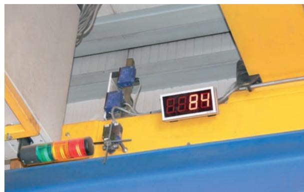
Technological weighing and displaying the actual load weight on the large-screen 4-5-6 digit display. Accuracy of weighing in dependence on an used tensiometer 1-2% from nominal capacity (or less).
