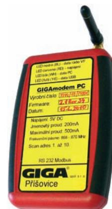
Radio modem GIGAmodem PC. One Master modem connected to PC can communicate with up to 10 SLAVE modems installed on cranes which can be remote up to 1,0 km.
